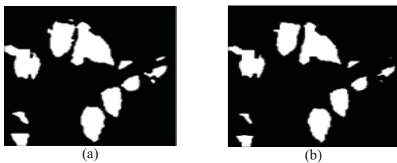
Fig. 4. The Output example of image morphology process for Data 1: (a) Closing, (b) Opening
